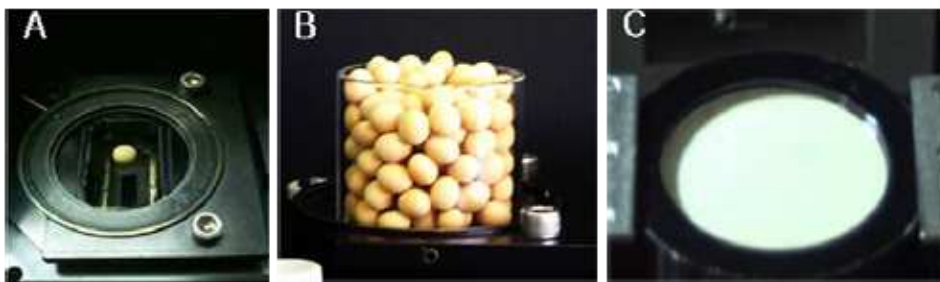
Fig. 4. General shape of soybeans, single seed (A), bulk seeds in cup (B), and soybean flour (C) for spectra collection.
