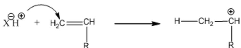
Scheme II. Formation of a carbocation by the attack of a proton on the olefin double bond
